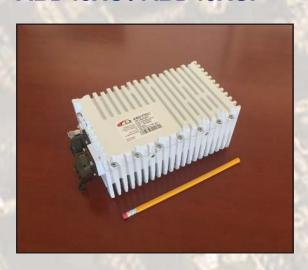
This smallest and lightest 40W L-To C-Band Block Up Converter is based on GaN technology. It is designed to be mounted on the feed horn. The unit covers all three C-Band sub-bands: Standard (5.850-6.425 GHz) and Palapa (6.365-6.725 GHz) and Insat (6.725-7.05 GHz).
