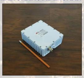
This smallest and lightest 10W L-To Ku-Band Block Up Converter is based on GaN technology. Double L.O. and field-exchangeable connector make unit universal for any Ku-Band application. Incomparable low power consumption allowes the BUC to be powered by iDirect and similar modems. Internal 10MHz reference option enables using the BUC with the modems without 10MHz reference.
