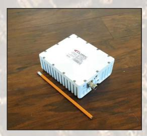
This smallest and lightest 8W L-To C-Band Block Up Converter is based on GaN technology. It is designed to be mounted on the feed horn. High power efficiency resulting in the low current (<1.15 amps @ 24VDC). The unit covers all three C-Band sub-bands: Standard (5.85-6.425GHz), Palapa (6.365-6.725 GHz) and Insat (6.725-7.05 GHz).
